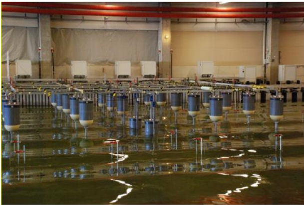
Figure 5: Impression of a 2-WEC column array under regular waves, (V. Stratigaki, et al., (2014))
