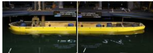
Figure 31: Photo of load variation test on design draft condition
