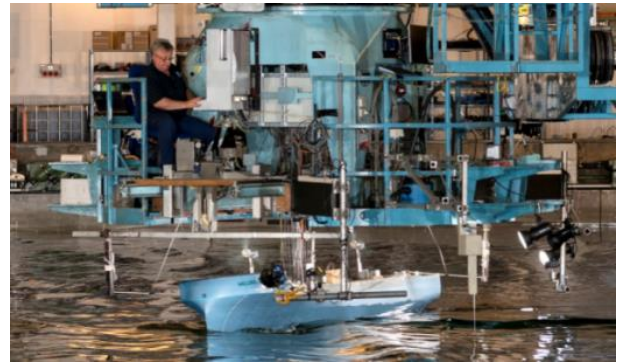
Figure 11. Wave tests with a model of Oceanbird ( the wing sails have been replaced by fans/airscrews) ( F C Gerhardt et al. , 2021)
