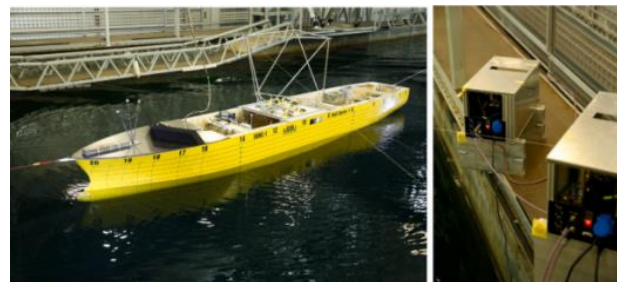
Figure 12. Model of SOBC-1 in the towing tank (left). Two of the six actuators mounted on the car-riage (right).( Sauder and Alterskjær , 2022)
