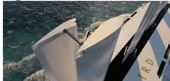
Figure 1: Top view of a rigid wing-sail from the Oceanbird concept (Oceanbird 2023).
