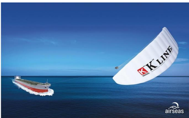
Figure 3: Towing kite - Airseaks L Line https://airseas.com/
