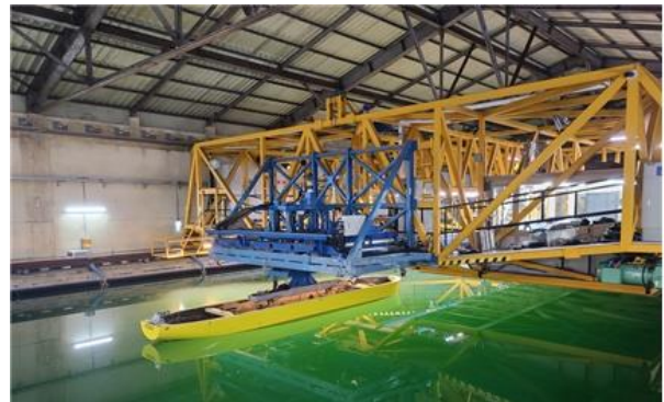
Figure 35: Photo of static drift test on heavy ballast condition
