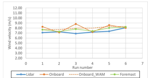
Figure 59 Wind velocity measurement results at each anemometer position during speed trial of a LPG carrier in stable wind
