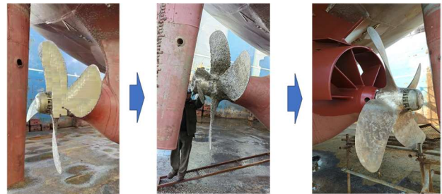
Figure 90 Carried out multiple exchange of ESDs on “Mid-scale” test ship
