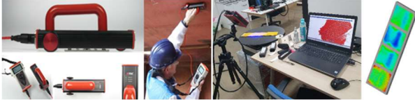
- Contact Type - - Non-contact Type - Figure 11 Hull roughness measurement system
