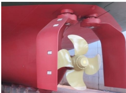
Figure 27. Gate rudder system of Shigenobu.
