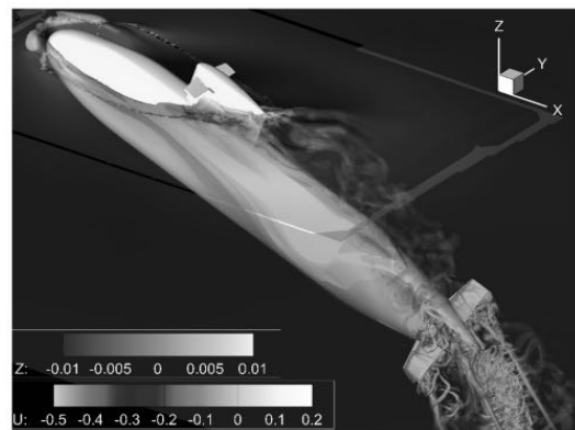
Figure 35. A submarine manoeuvres at a large pitch angle after breaking the surface. Vortical structures are shown as isosurfaces of Q = 3000 coloured with axial velocity.
