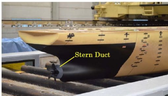
Figure 25. Stern duct on Japan Bulk Carrier.
