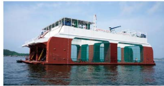
Figure 111: Semi-submersible aquaculture platform "Penghu" (Ding et al. 2023)
