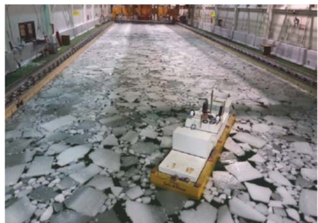
Figure 59: View of the ice basin and the model DP vessel
