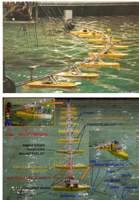
Figure 35 Hydroelastic bridge model and instrumentation (Rodrigues et al., 2022)
