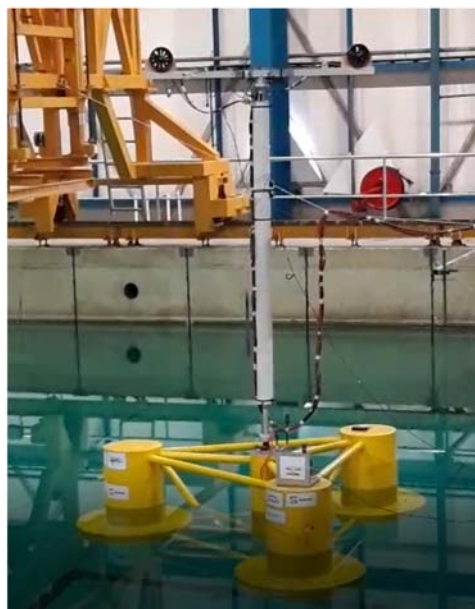
Figure 85: Model in the BGO FIRST basin (Cinello et al., 2022)
