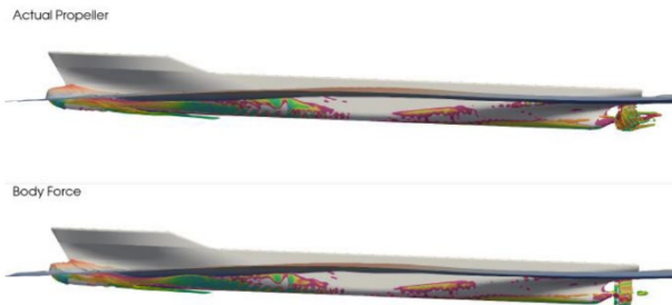
Figure 45: Vortical structures around ship hull. Above: actual propeller. Below: body force propeller, (Wang et al. 2023b).
