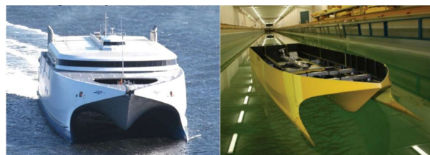
Figure 51: Incat Tasmania 112 m wave piercing catamaran 'Express 1' and 2.5 m model in towing tank (Lau et al. 2023a).
