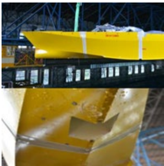
Figure 17: Model and bow opening used in the investigations of Chen and Wu (2021).
