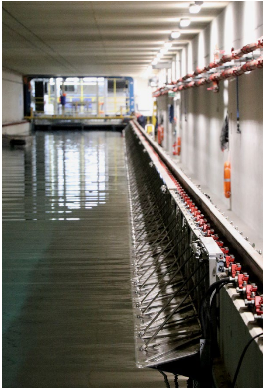
Figure 1: View of the deployed automatic side beach at Boldrewood towing tank (Malas et al. 2024).
