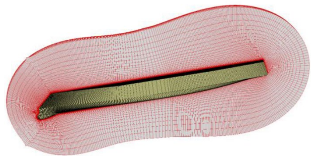
Figure 46: Body-fitted mesh used in the overset solver, Wu et al. (2022).
