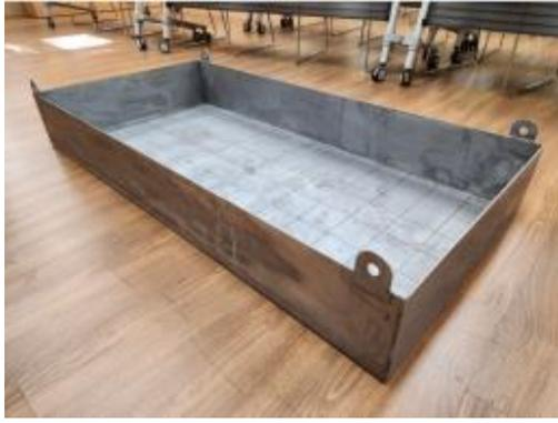
Figure 67: Stiffened plate fabricated for validation tests.
