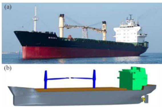
Figure 70: Test (a) and simulation (b) geometry model of general cargo vessel REGAL; (Song *et al.*, 2021)
