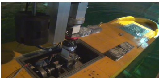
Figure 3: Ship model of C11 Containership in partially restrained experiment (Bu et al. 2019)
