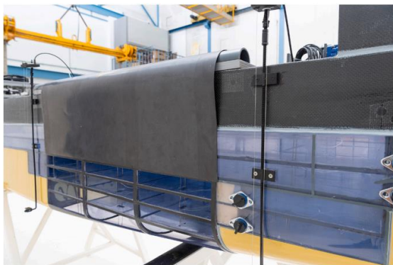
Figure 10: Breach opening and the magnetic cover (photo courtesy of MARIN)
