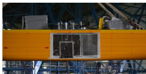
Figure 44: Self-designed electrically operated valve for controlling the opening's size
