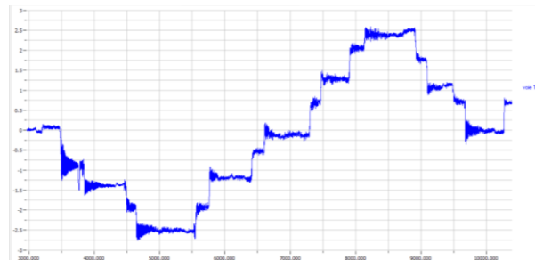
Figure 30: Heel measurement during an IT (3 hours), with gust wind effect visible, from Leguen et al (2023).
