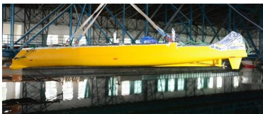
Figure 4: Ship model of ONR tumblehome hull in partially restrained experiment (Bu et al. 2021)
