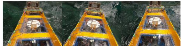
Figure 14: Movement of deck water due to ship roll with a phase lag for one of the irregular wave trial, Froude number 0.3 with open openings
