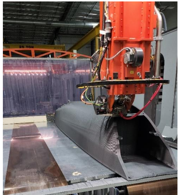
Figure 88. Angled Layer Printing (ALP) LSAM Model 5796.
