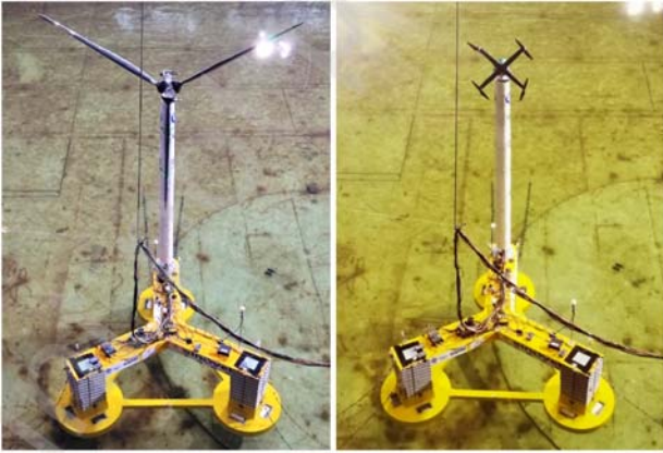
Figure 73: The presence of a full physical model and hybrid model in the experiment (Wen et al., 2022)
