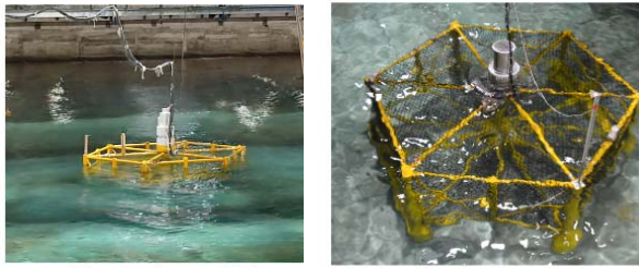
Figure 107: Physical model of the floating aquaculture platform in operational (left) and extreme bottom-sitting (right) conditions (Yu et al. 2023)
