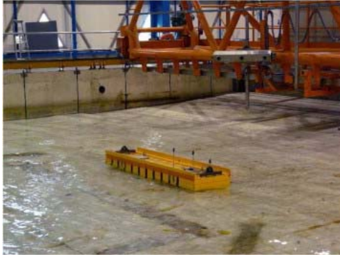
Figure 201: Barge model undergoing irregular wave tests at the shallowest position (Liu et al. , 2011)
