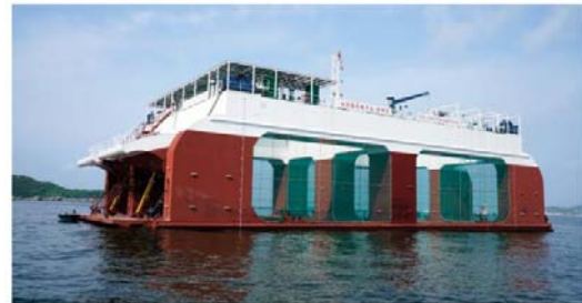
Figure 111: Semi-submersible aquaculture platform "Penghu" (Ding et al. 2023)
